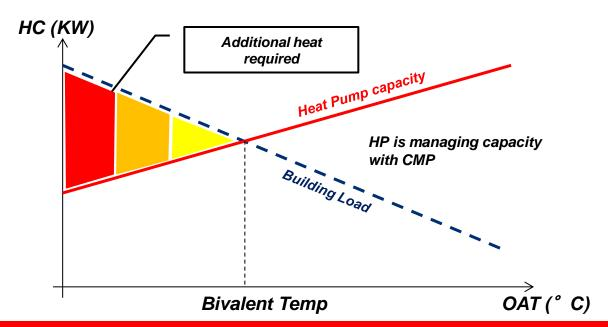
CXAX remains the main source of heating But coordinate with other heating sources
