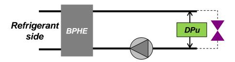
Customer shall prevent evaporator freezing by implemented a solution to guarantee a minimum water flow through the evaporator.
